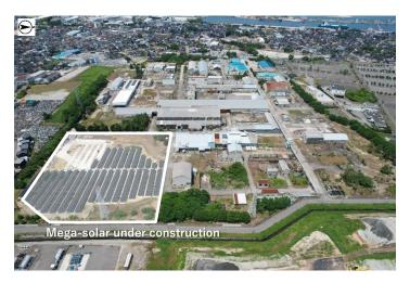
A 900kW solar power plant (mega-solar) is currently under construction in the southeastern part of the factory grounds, and is scheduled to be completed at the end of 2024. With the completion of this facility, all solar power generation facilities on the factory grounds will be able to generate 1 MW of electricity.
